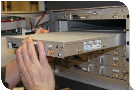
Figure 4. Power modules simply slide into the power block and join both electrical and leak-free cooling connectors. Two panel screws secure the power module.
