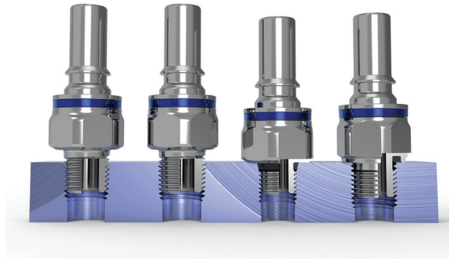
Left to right: NPT, BSPT (R), SAE ORB, BSPP (G)
